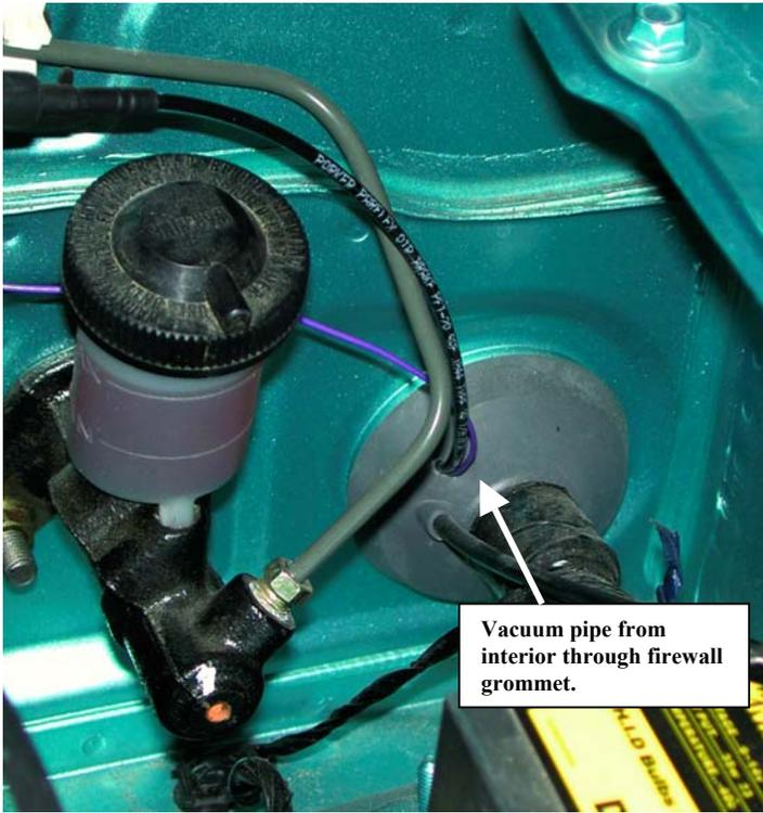
2. Route the hard plastic pipe across the back of the engine and across the valve cover. Connect this hard plastic pipe to the vacuum fitting on the intake manifold with the small, 90-degree adapter hose. Connect the other end to the Jackson Racing PowerCard by sliding the hard plastic pipe into the silicone hose of the PowerCard.
