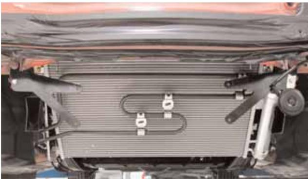
7. Gather the oil cooler, the four remaining M6 bolts, and the four M6 lock nuts. Bolt the oil cooler to the oil cooler brackets that were installed in the last step. Slip the bolts through the oil cooler first then the brackets and finally, start the nuts on the back side. The fittings should be on the drivers' side of the vehicle with the 90 degree fitting on the top. Tighten all six M6 bolts to 6ft. lbs. Now tighten the bumper bolts to 18 ft. lbs. Illustration 7.
