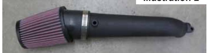
3) Test fit the CAI assembly to the car. Adjust the filter as necessary to make it clear the body of the car.
