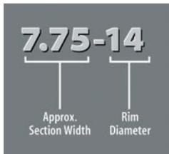
Numeric sizing was the standard through the late-sixties. Section widths ending in zero were 92-series, and 82 aspect ratios were indicated by section widths ending in numbers other than zero. (Courtesy Yokohama)
